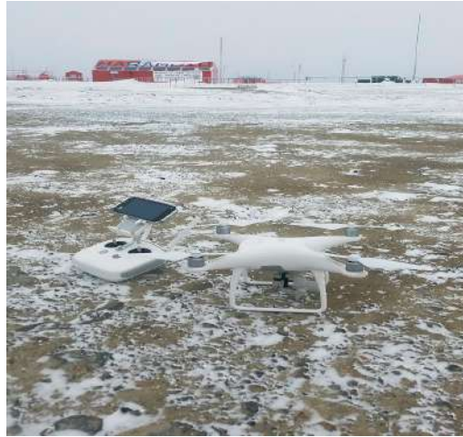
Foto N° 11: VANT Marca DJI, modelo Phantom 4 Advanced.
